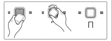
After changing the filter, push and hold the Air Filter button for three seconds to reset the filter sensor.
